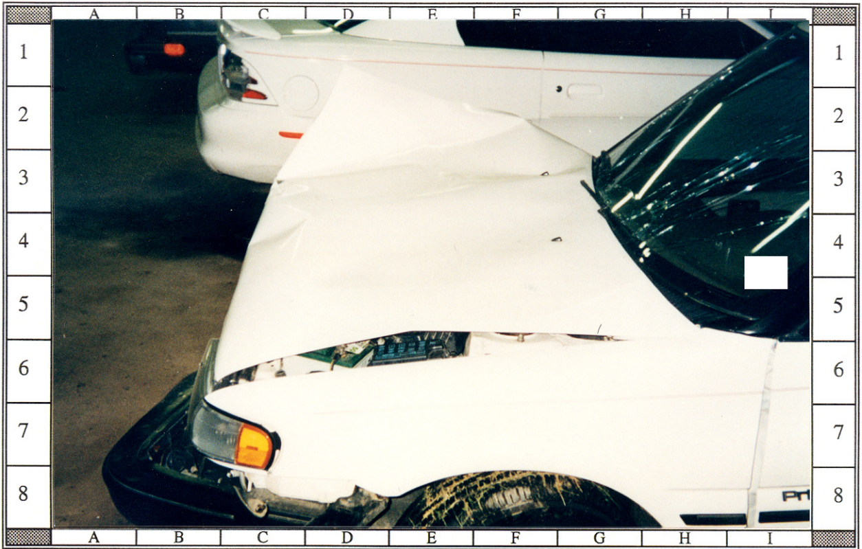
# 15: Vehicle #2's frontal crush viewed from left showing slanted front bumper and induced damage to hood, left fender, and windshield
